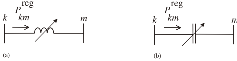
Figure 5.9 Thyristor-controlled series compensator equivalent circuit: (a) inductive and (b) capacitive operative regions
